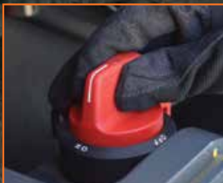
Battery cut-off switch
