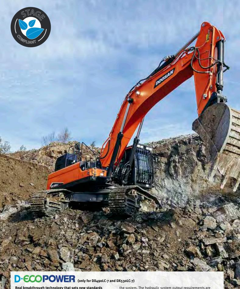
Real breakthrough technology that sets new standards in the industry: The exclusive ECO Power system improves productivity and saves fuel. A pressure-controlled pump, closed-center main control valve, and 9 sensors electronically detect and control the precise amount of hydraulic oil required to perform a task. The exact amount of oil required is metered instead of continuously forcing a fixed amount of oil through
