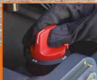
Battery cut-off switch
