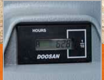
Hour meter (from ground level)
