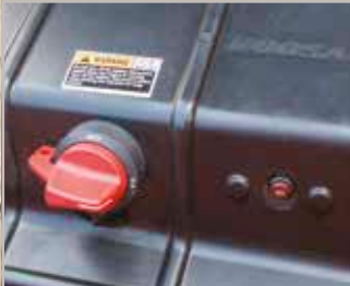
Battery cut-off switch
