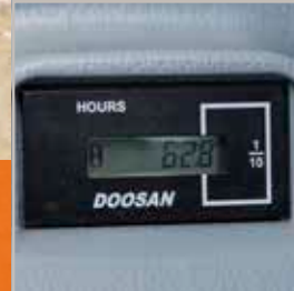
Hour meter (from ground level)
