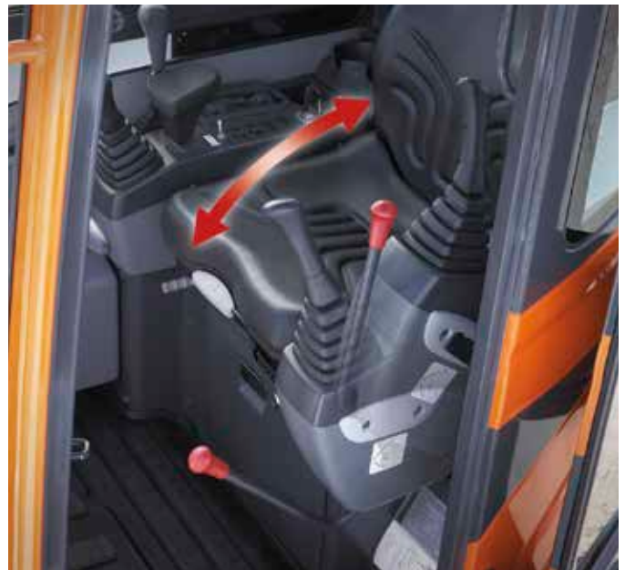
Control stand tilting function
