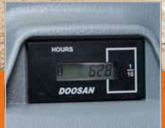
Hour meter (from ground level)
